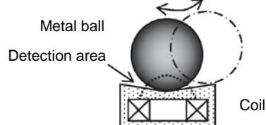
\*4. Whether the metal ball built in the sensor is detected or not determines the ON/OFF state of the output transistor. (Intermittent output)
