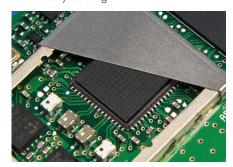
Gap Pad® EMI 1.0 is a highly conformable, combination gap filling material offering both thermal conductivity performance and Electromagnetic Energy absorption (cavity resonances and/or cross-talk causing Electromagnetic Interference) at frequencies of IGHz and higher.
