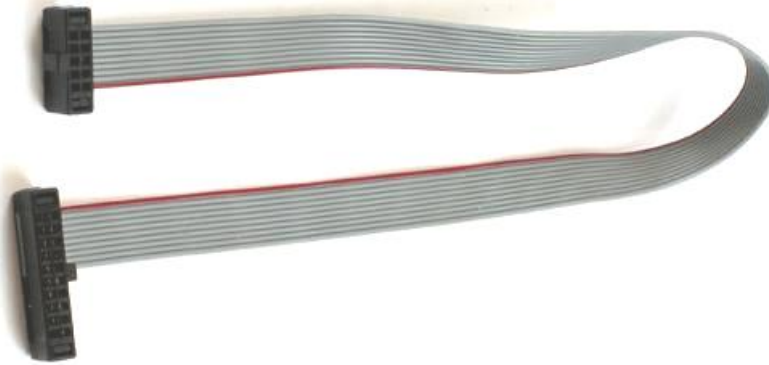
Figure 6 – 10-pos to 20-pos Debug Cable
