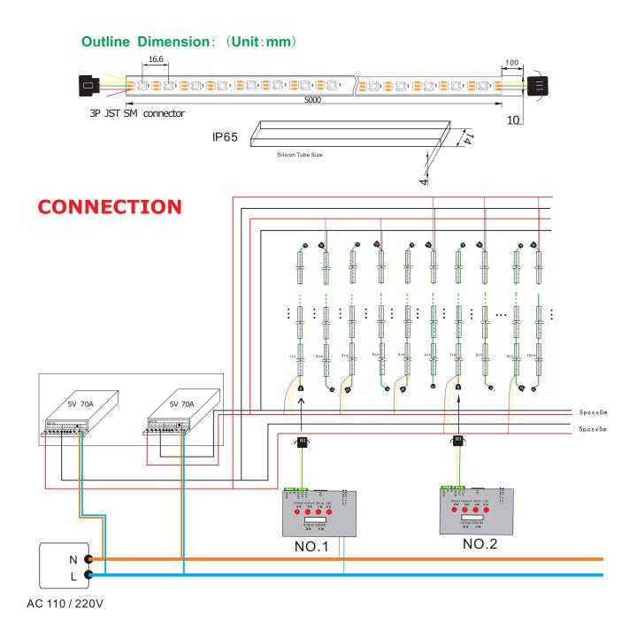
This strip 60Pixels (IC) per m,5m/roll (300Pixel),T-1000controller support 2000Pixel Max, 1 Roll strip total power is 72W (5m),each 5V70A(350W) works 4rolls of strip . You also could use T4000、T8000 SD controller for more LED pixels
